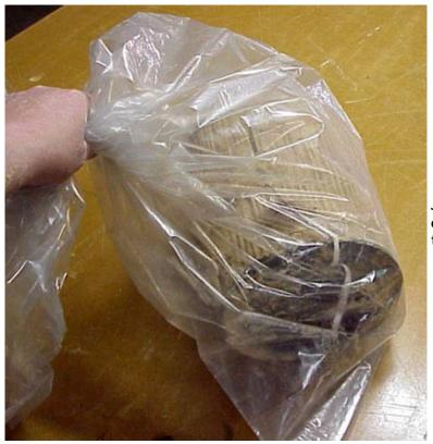
Just place the filter inside a garbage bag and tap on the workbench. Rotate the filter while tapping to make sure you clean all of the folds. In no time at all the filter is clean and all of the dust is inside the bag.
